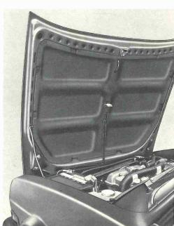
The hood is held in open position by the rod. Illumination of the engine compartment is by a light under the hood. It operates automatically when the hood is raised and the parking lights are on.
