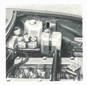
Every 5,000 miles, check level of antifreeze in the reservoir; this should be done exclusively with a cold engine as with a hot engine the level may increase remarkably, even after stopping the engine. The level of mixture in the reservoir should never fall below the « Min » nor exceed the « Max » marks. To top up use Alfa Romeo Antifreeze suitable for aluminum alloy engines
