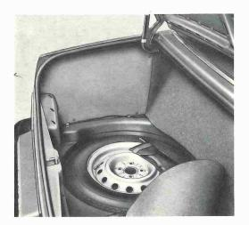
The spare tire and the tool kit are in the trunk under the mat.
